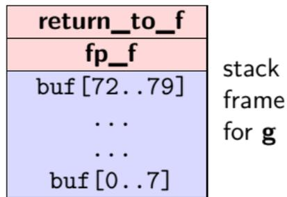
in **g()** we overflow **buf** to overwrite frame pointer **fp\_f** with **fp\_g**.
