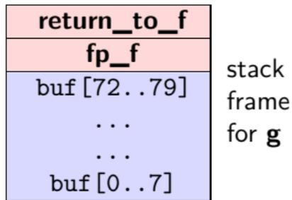
in **g()** we overflow **buf** to overwrite the return address **return\_to\_f** to point in **some code somewhere**, and the framepointer to point inside **buf**.
