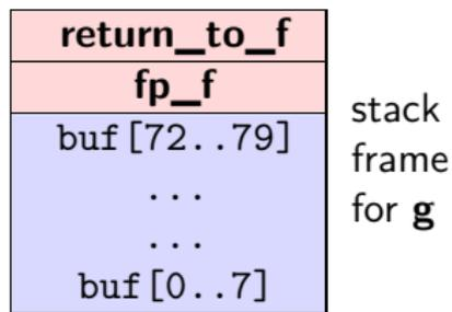
in **g()** we overflow **buf** to overwrite frame pointer **fp\_f** with some pointer into **buf**.
