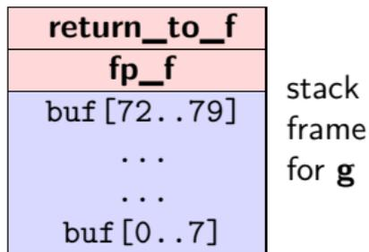
in **g()** we overflow **buf** to overwrite the return address **return\_to\_f** to point inside **buf**
